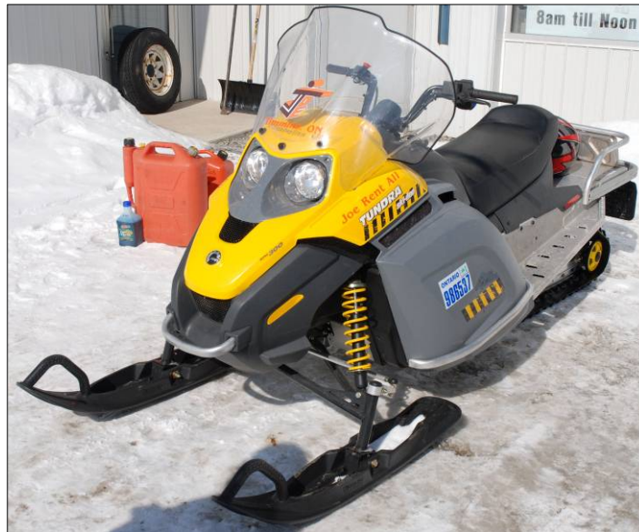
Figure 2: View of the test snowmobile (2007 Ski-Doo Skandic Tundra 300).
